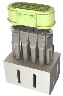
TELSONIC's ultrasonic tools weld pieces together by using vibration oscillations to generate intramolecular frictional heat, and the company's engineers rely on SOLIDWORKS Simulation Professional software to quickly run modal analyses and predict frequency modes with a high degree of accuracy to support this process.
