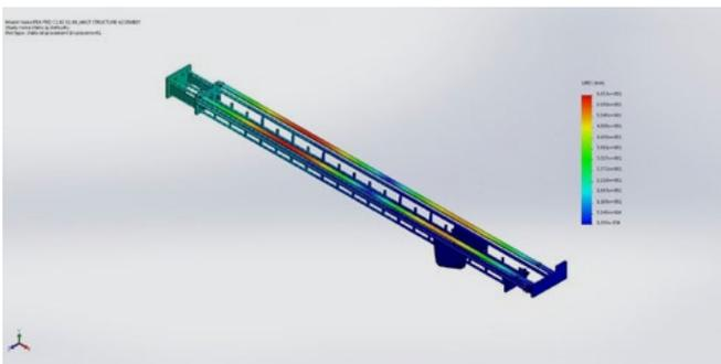
With SOLIDWORKS Simulation Professional structural analysis software, Paranthaman Exporters can conduct both part and assembly FEA studies to validate rig performance. This capability enables the company to improve the strength and performance of its equipment while decreasing rig weight and reducing material usage and associated costs.
